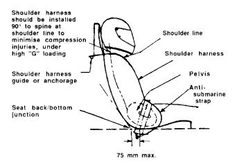
75 mm max, to centreline of lap belt at seat back/seat bottom junction. Lap belt should continue in straight line to anchorage.
